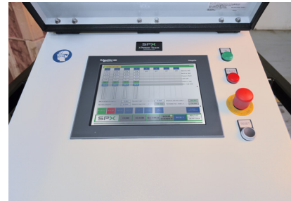
The home screen on the Motion Control System is easy to use and operate. It highlights all activities during use of the Motion Control System. For each cylinder in operation, the cylinders performance is captured and displayed on the HMI screen as illustrated below.
